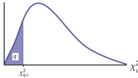
Figure 2.82: Illustration of the probability calculations for \chi^2 distribution with k degrees of freedom. The value \chi^2_{q,k} is such that a total probability of q is enclosed in the left tail of the distribution.
